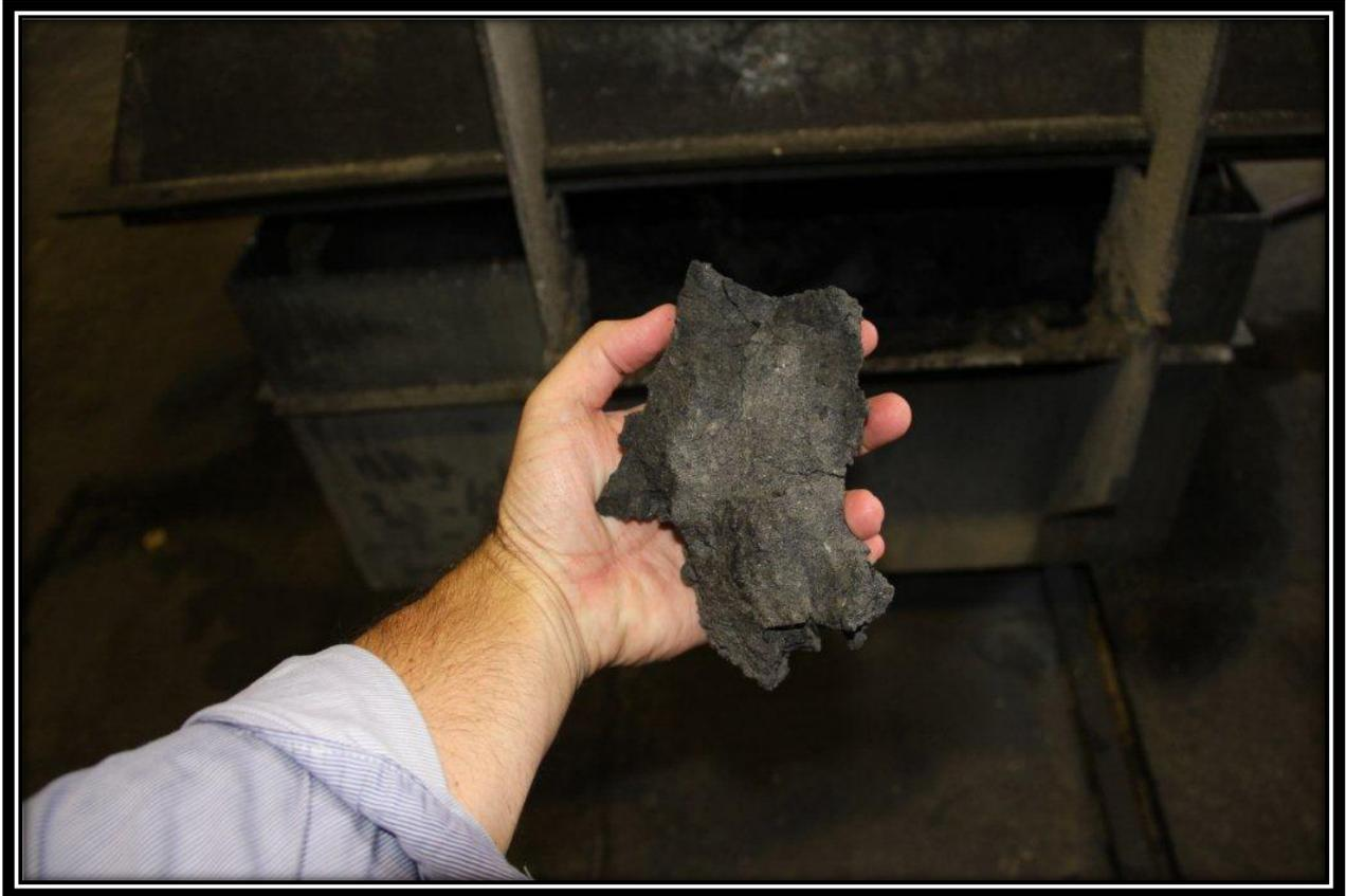
*Figure 3: Coke Produced from the Pilot Oven Before Mechanical Strength (drum index) Tests*
