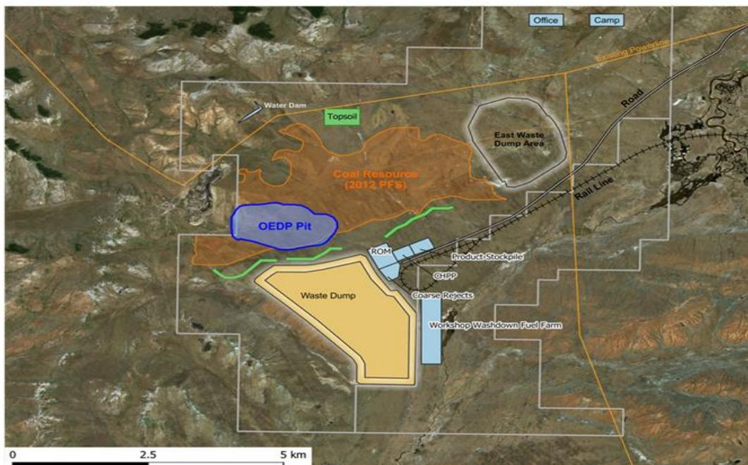
**Figure 2: OEDP pit plan within the overall layout**
