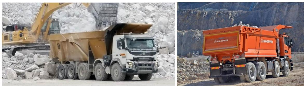
*Figure 1: BAS Mining 10x4 Tipper (Left), Scania Mining G500 8x4 Tipper (Right)*
