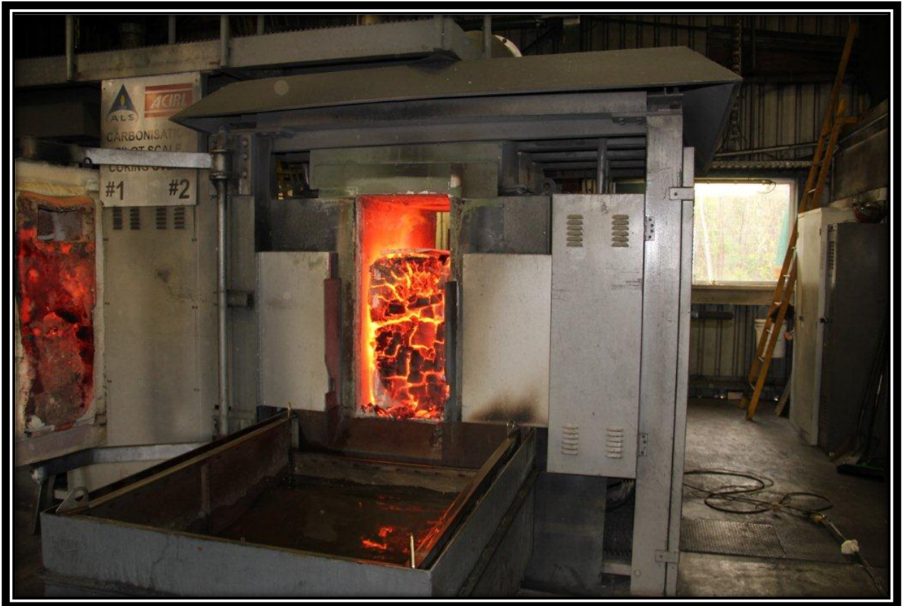
Figure 1 Coke Produced Using 100% Indicative Ovoot Coking Coal Just Prior to Coke Push and Quenching.
