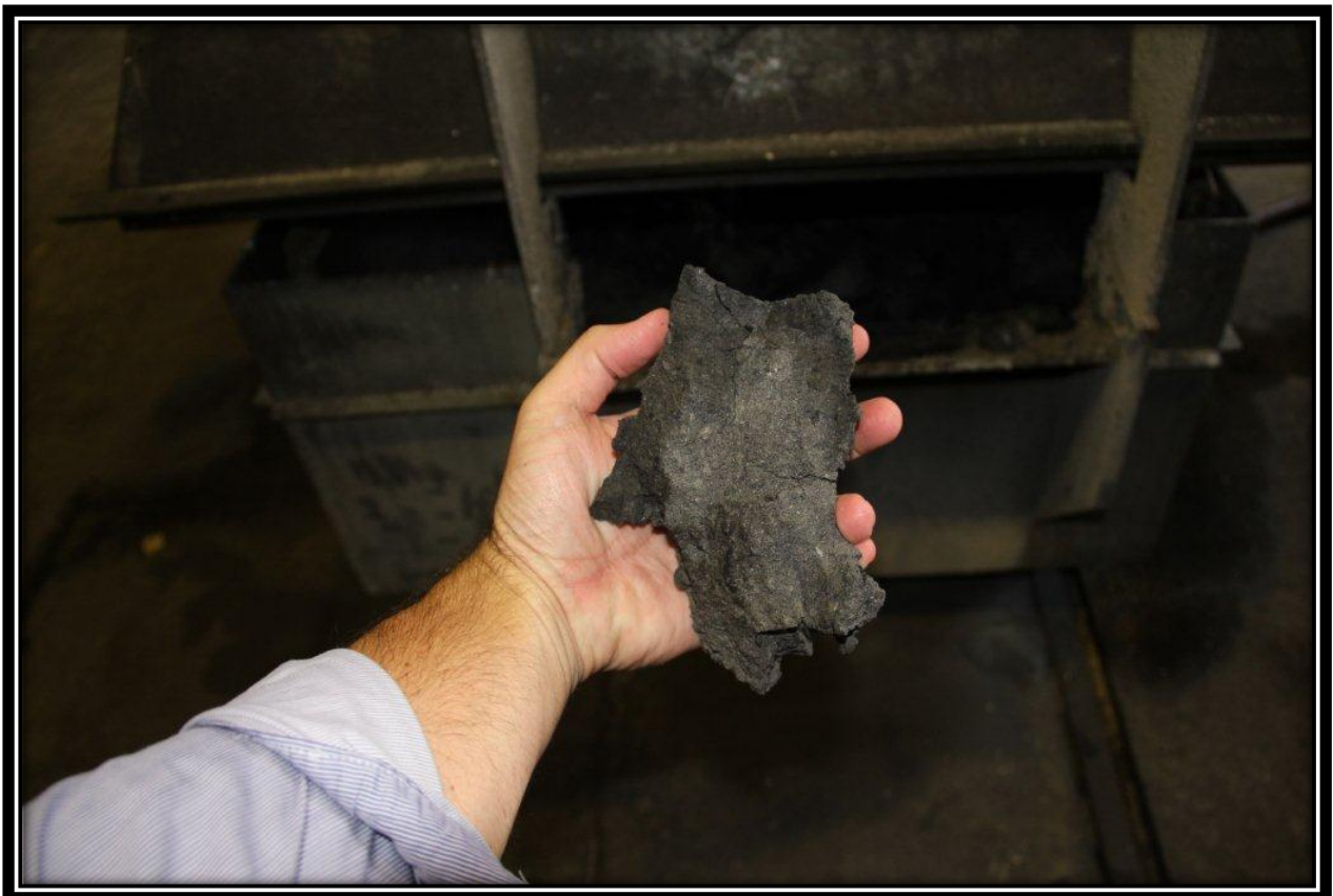
Figure 2: Coke Produced from the Pilot Oven Before Mechanical Strength (drum index) Tests
