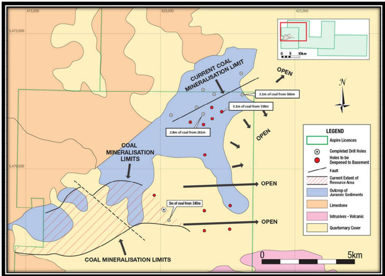
**Figure 1: Drill Hole Location Plan - exploration holes completed and to be deepened**
